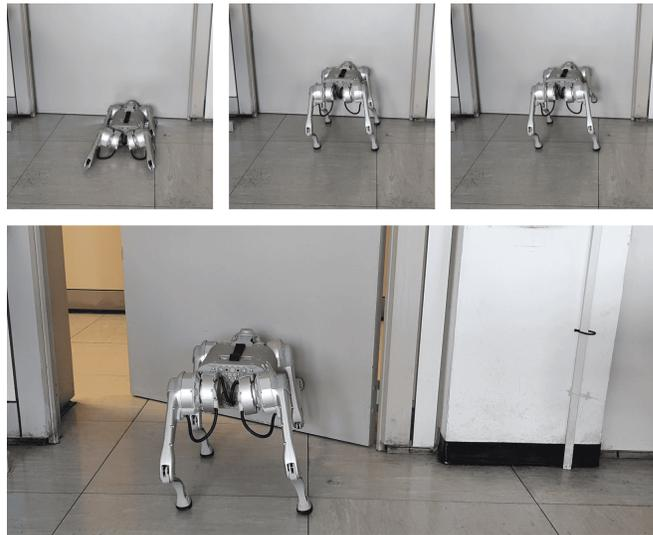
Fig. 6. The robot uses the front right leg to opens a half-closed door, making it possible to pass.
